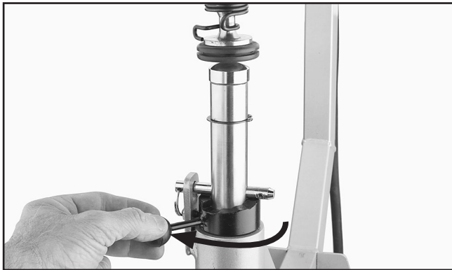
Figure 11. Raising the die up closer to the hammer using the die housing lever.
